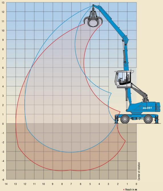
Work equipment: Box-type boom 6.5 m;
